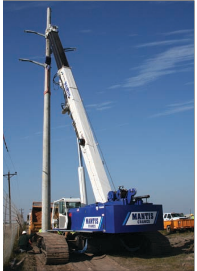
The ability to telescope the boom under full load simplifies the handling and placement of heavy concrete poles.
