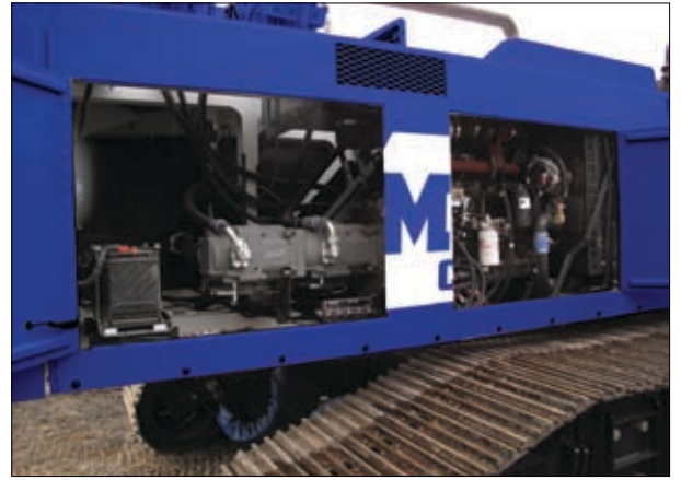
Large access doors, spacious machinery compartments simplify preventative maintenance and service of the crane.
